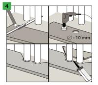
Act similarly in the case of a bigger number heating system pipes. The cut panel elements must be joined with the assembly adhesive for plastic elements.
