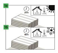
If the temperature is >5 °C during transport, the acclimatization time in a room with a temperature of 18-30 °C should be min. 24 hours. However, in case of temperature <5 °C during transport, acclimatization time in a room with a temperature of 18-30 °C should be min. 48 hours.
