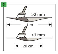
Make sure that the substrate is completely flat. All substrate irregularities exceeding 1 mm, with a length greater than 20 cm, or exceeding 2 mm with a length greater than 1 m must be levelled. Check if the use of the priming or sealing material is necessary. In order to prepare the substrate perfectly, spread the grout or the self-levelling compound on the entire surface.
