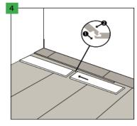
The Afirmax floor panels are provided with locks on the short and long side. First, connect the panel on the long side; for this purpose slide the long side of the panel into the groove of the previously installed row of panels. Move to the corner, leaving some clearance.
