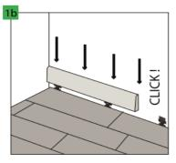
Expansion joints along the walls must be covered with a decorative strip, assembling it by means of glue or special clips. It is recommended to use the Arbiton strips dedicated to a given panel, which guarantee the excellent colour match and the coat resistant to scratching.
