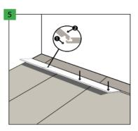
Then lower the panel in such a way as to fasten the lock on the short side, gently pressing the panel with fingers, starting from the corner and then towards yourself. The lock on the short side is provided with a special catch, which gets snapped if properly assembled. NOTICE! Do not use excessive force! If there are any difficulties with the lowering of the panel and closure of the lock, increase the clearance in the lock and lower the panel again.
