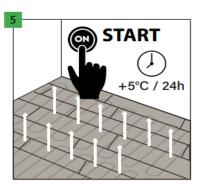
After laying the floor and waiting 24 hours, you can turn on the underfloor heating, remembering to gradually increase the temperature (5°C per day). ATTENTION! It should be remembered that the maximum temperature of the floor surface is 27°C.
