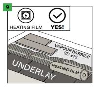
Installation on a heating foil is also allowed, provided that an appropriate underlay for the heating film and a vapor barrier foil SD ≥75 are used.
