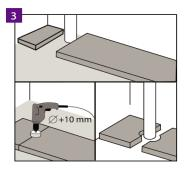
In the case of vertical pipes embedded in the substrate, leave free space around the pipes. Holes for the pipes must be drilled with a drill bit with a diameter that is bigger than the pipe diameter by 5 mm.
