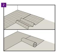
Make sure that the substrate is properly prepared. Then lay the Arbiton or Ewifoam brand underlay, which is designed for installation of rigid and LVT floors. The neighbouring ribbons of underlay must fit tightly and must be joined by means of an overlap or Arbiton or Ewifoam AluTape, without leaving any redundant space.
