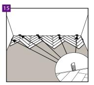
Leave 5 mm of perimeter space at the walls to allow the floor expansion. The maximum surface which can be laid without additional expansion joints is 200 m2. Above this surface, apply an additional expansion joint and enlarge all the expansion joints up to 10 mm. The maximum length of the floor surface in one direction, which can be laid without additional expansion joints is 20 m. Above this length, apply an additional expansion joint and enlarge all the expansion joints up to 10 mm.
