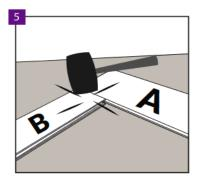
Then put panel A. Then connect panel B to panel A using a rubberized hammer. Note! Each panel contains only 1 lock that can be pinned down. Other locks must be installed without driving in (see installation, Figure 4). Note! Try the lock very carefully before driving in (lack of precise fit of the lock and then driving the panel in will cause its damage, which will result in rejecting a possible claim).
