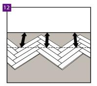
After laying four full rows of panels. Set the line along which the floor will be cut so that the resulting fragment can be moved towards the wall.
