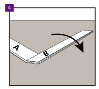
Mount (jam) without driving panel B in with the movement indicated in the figure above.
