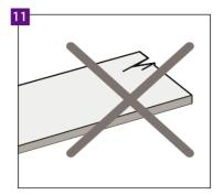
Before and during the installation, control all the panels in the optimal lighting conditions. Do not use defective panels.
