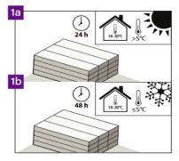
If the temperature is >5 °C during transport, the acclimatization time in a room with a temperature of 18-30 °C should be min. 24 hours. However, in case of temperature  $\leq$ 5 °C during transport, acclimatization time in a room with a temperature of 18-30 °C should be min. 48 hours.
