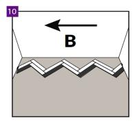
It is important that the assembly of each row is carried out with the principle that we assemble panels B to the left, i.e. the opposite direction of the assembly of panels A.
