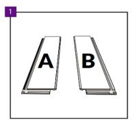
Each package contains two types of panels: A and B. The individual panels are marked at the bottom as A or B for easier differentiation. Parts A and B must be sorted separately before the installation. During installation, it is very important to ensure that panels A and B are installed at the right places in the row (see -> panels laying, point 7; 9 and 10).
