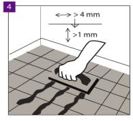
In the case of installation on the substrate covered with ceramic tiles, fill the tile joints with the gap wider than 4 mm and deeper than 1 mm with a durable compound for the filling of points, e.g. resin grout. Installation is allowed on tiles with grouts not wider than 5 mm and 1 mm deep without using levelling compound, provided the Multiprotec Super Hardlay or Vinclic Super Solid are used as underlay.
