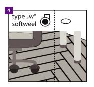
Used office chairs with W-type castors, protecting the floor additionally by means of the protective net. The furniture legs must be provided with protective pads which provide protection against scratching, e.g. made of felt.
