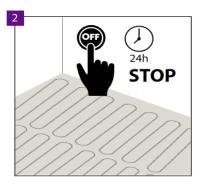
Before installation, turn off the underfloor heating for 24 hours.
