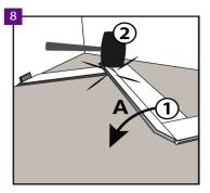
Laying of the second row should also be started with panel A. Please keep the rules in mind at all times concerning installation of the panels – when driving panel B in to panel A, the long sides are installed by jamming, while the short sides are assembled by driving in.
