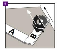
Install next B panel in the same row (see floor installation manual – Fig. 4). Cut the panel making sure to use proper wall expansion joints (see floor installation manual – Fig. 15).
