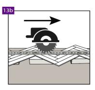
When cutting, we recommend using spacers that must be placed under the floor to avoid damaging the underlay. The height of the spacers should be adjusted according to the guidelines specified by the manufacturer of the circular saw or guide saw.
