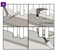
Act similarly in the case of a bigger number heating system pipes. The cut panel elements must be joined with the assembly adhesive for plastic elements.
